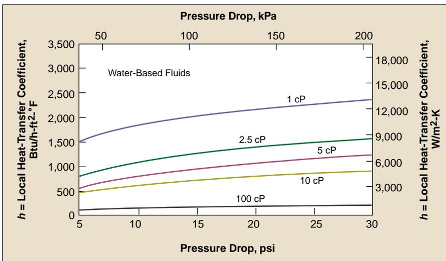
Figure 4. Heat-transfer correlations for water-based fluids,  $4.0 < NTU < 5.0$ .
