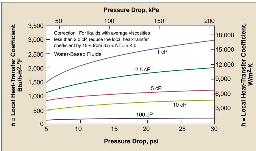
Figure 3. Heat-transfer correlations for water-based fluids,  $2.0 < NTU < 4.0$ .
