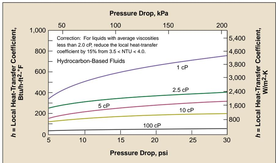
Figure 6. Heat-transfer correlations for hydrocarbons,  $2.0 < NTU < 4.0$ .
