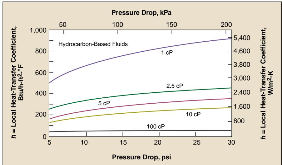
Figure 5. Heat-transfer correlations for hydrocarbons,  $0.25 < NTU < 2.0$ .
