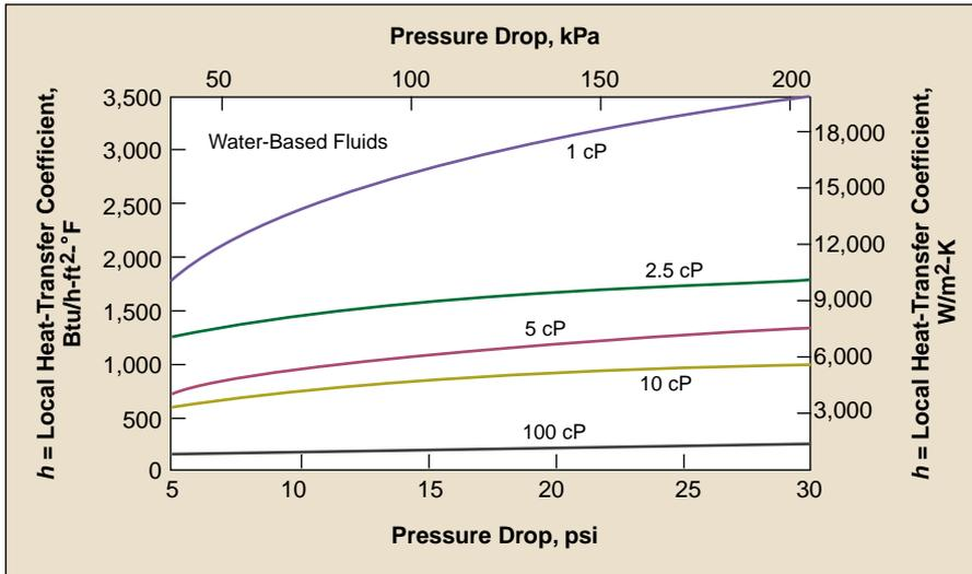
Figure 2. Heat-transfer correlations for water-based fluids,  $0.25 < NTU < 2.0$ .
