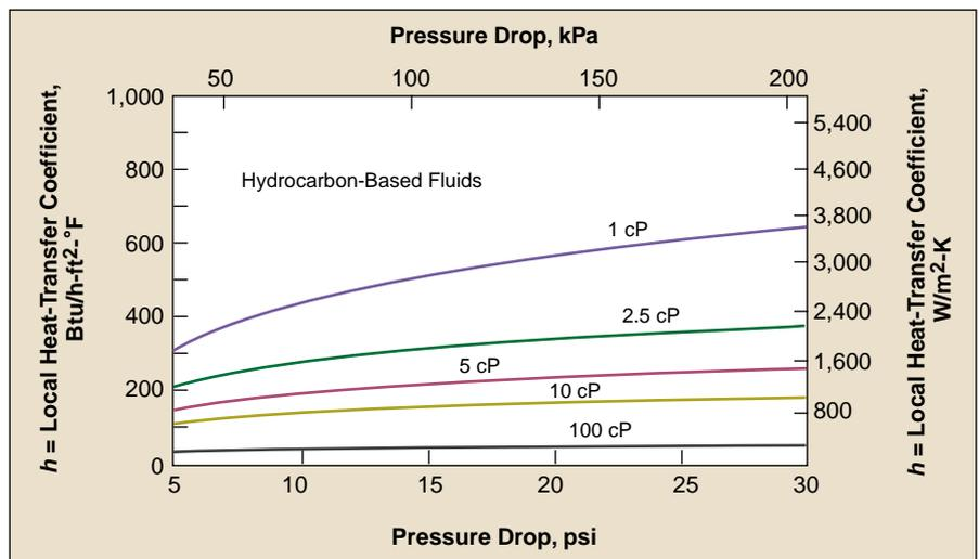
Figure 7. Heat-transfer correlations for hydrocarbons,  $4.0 < NTU < 5.0$ .
