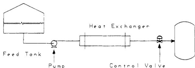
Figure 1. Process for pump and control valve design.
