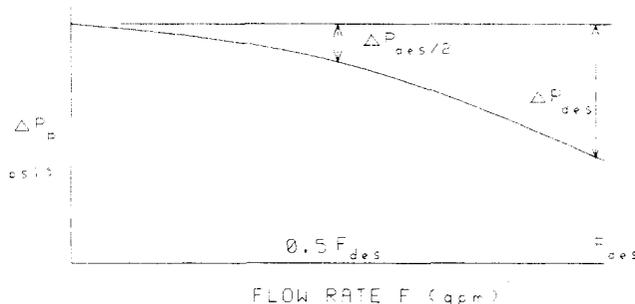
Figure 2. Parabolic pump curve.
